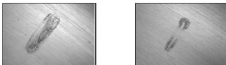
Figure 9: Comparison of the damages depending on the temperature (left 25°C; right -10°); Parameters: 750 N/ Ball; 25 Hz; \pm 0.5^\circ , 117000 LC; Li-Complex-Grease
