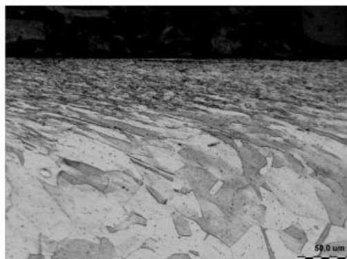
Figure 4: Microstructure of 316 LVM steel sheet after MPT. Light microscope
