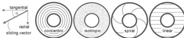
Figure 3: Specimen with applied directional and isotropic patterns (schematic)
