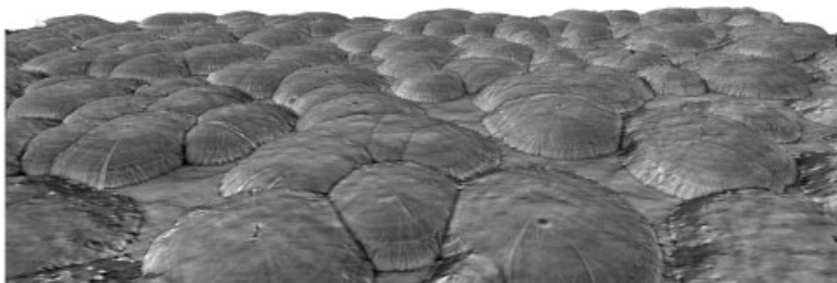
Figure 1: Electrochemically structured steel surface – 3D-SEM (here X13 CrMnMoN 18 14 3 after loading test)
