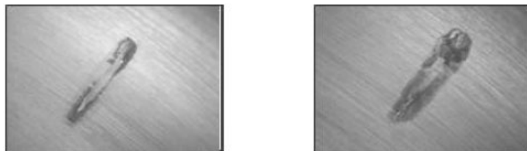
Figure 8: Comparison of the damages depending on the temperature (left 25°C; right -10°); Parameters: 750 N/ Ball; 25 Hz; \pm 0.5^\circ , 117000 LC; Ca-Complex-Grease
