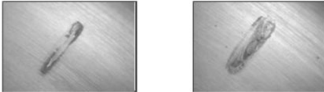
Figure 11: Comparison of the damages of greases with the same base oil and additives but different thickener (left: calcium complex soap; right: Lithium complex soap); Parameters: 750 N/ Ball; 25 Hz; \pm 0.5^\circ , 25^\circ\text{C} , 117000 LC
