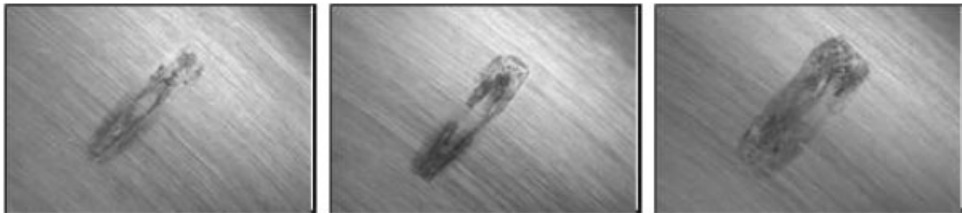
Figure 7: Increased damage with increasing frequency (left 5 Hz, middle 12,5 Hz, right 25 Hz) – Parameter: Low-Ref.-Grease, 750 N/ Ball; \pm 0.5^\circ , 25^\circ\text{C} , 117000 LC
