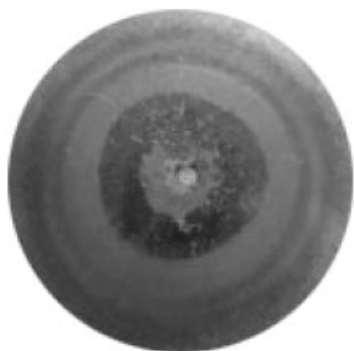
Figure 3: Example of a worn hardened specimen
