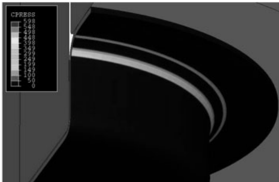
Figure 4: Computed distribution of contact pressure (MPa) during deep drawing operation on 0.5 mm AISI 304.
