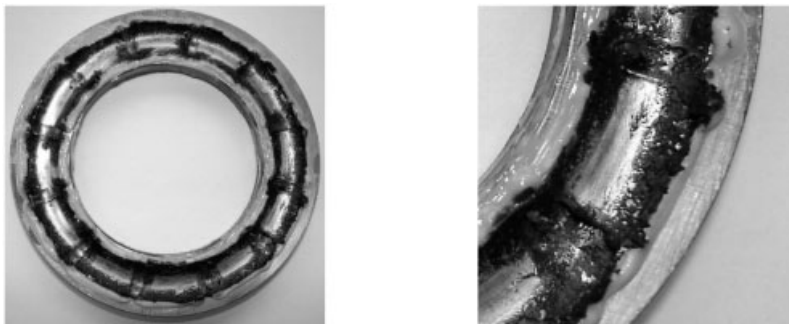
Figure 1: Axial bearing with advanced damage. Typically there are marks in the distance of the rollers.
