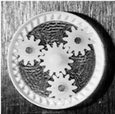
Figure 2: Photograph of the first micro planetary gear train (outer diameter \approx 5\text{mm} ) made of ceramics.
